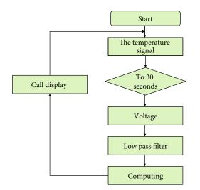
FIGURE 5: The structure diagram of the body temperature collection module.
