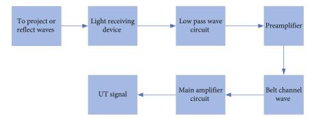
FIGURE 4: The pulse acquisition module diagram.
